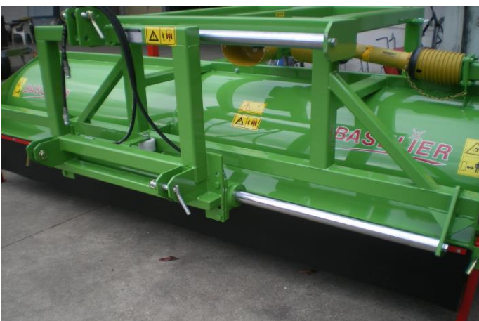
Hydraulic sideshift to move topper 1 row
