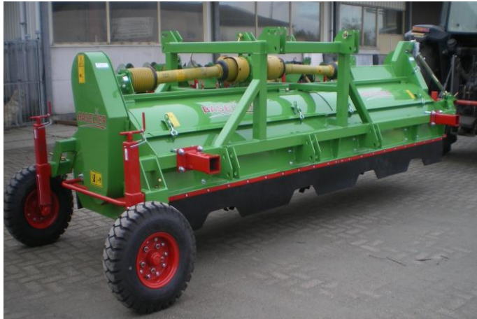
End tow kit by replacing the wheels
