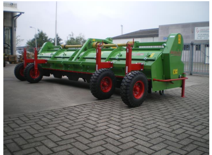
Standard 6LKB460 with 4 depthwheels
