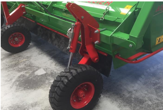
Hydraulic depthwheels instead of spindle
