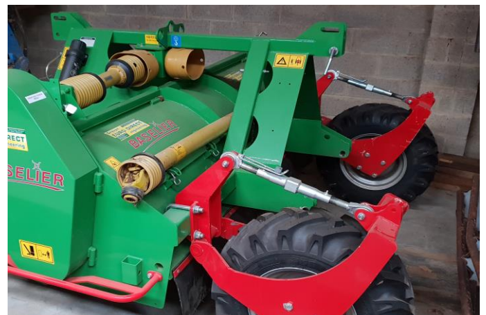
Wheel 10,0/75-15.3 instead of standard wheel
