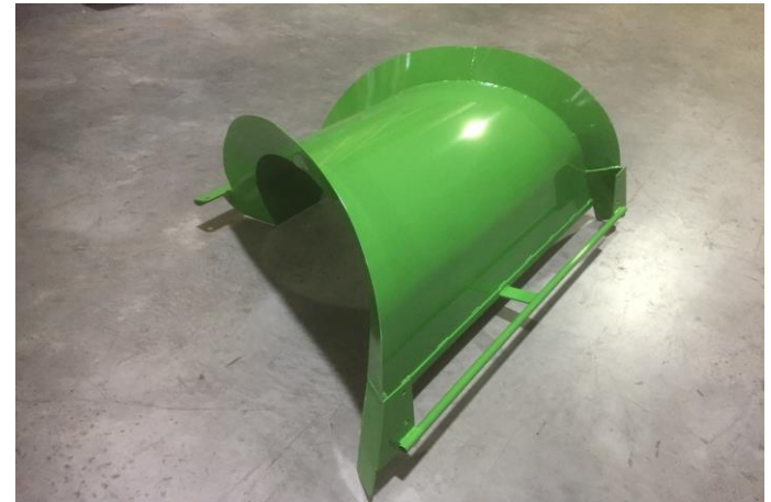
Centre plate to deflect haulm to wheeltracks
