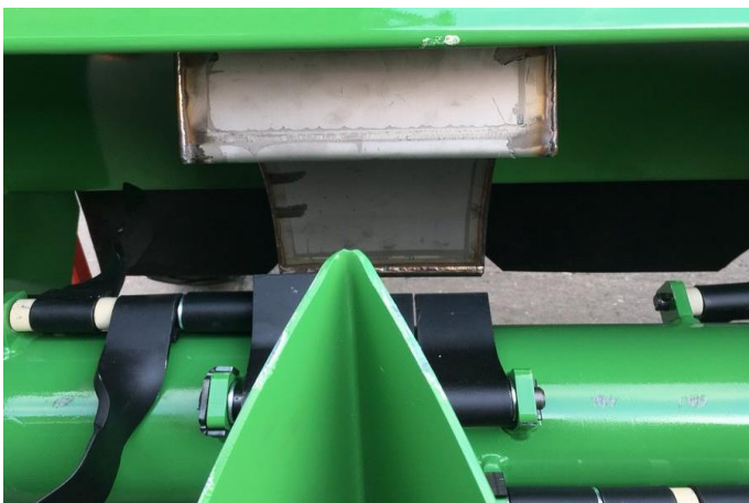
Haulmdeflectors in seedling (stainless steel)
