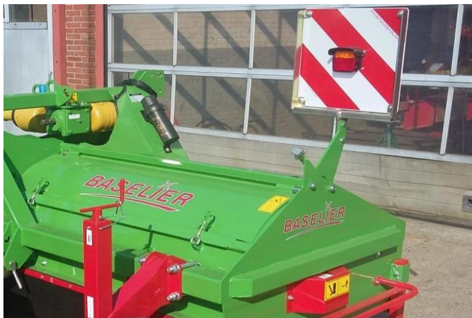
Led lighting and marking signs
